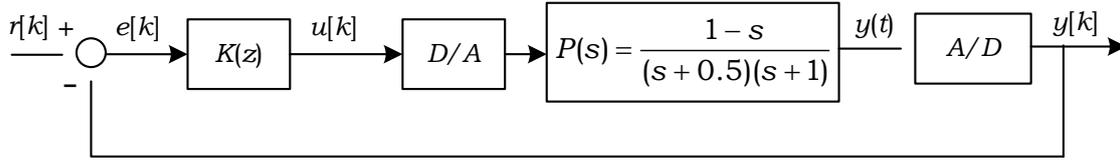
Applied combination of digital/analog D/A and analog/digital A/D conversion is modeled as zero order hold circuit and ideal sampling. Sampling period is  $T = \ln 2$  sec.
